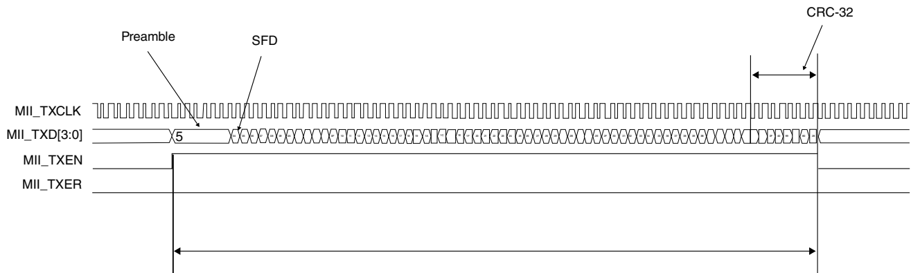
Figure 23-128. MII transmit operation
