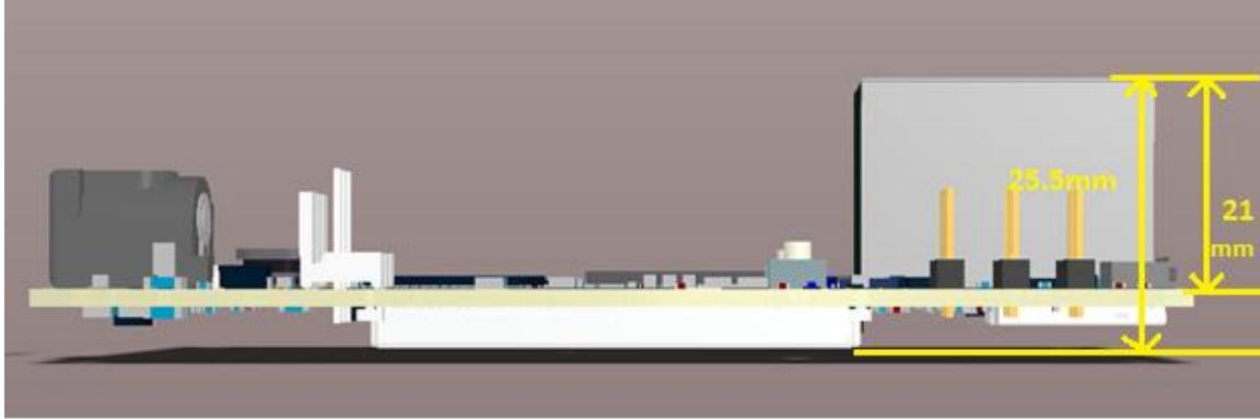
Figure 19 – MicroZed Side Vertical Dimensions
